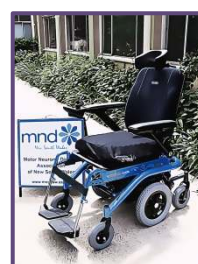
Figure 16 Electric tilt in space wheelchair
