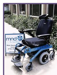
Figure 16 Electric tilt in space wheelchair
